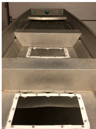
Installing the plexiglass viewing areas in our 'glass bottom boat' and the final installation
