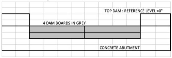
The dam master regularly measures water level from the reference level at the top of the concrete abutment. We have water level records going back to 1994.
